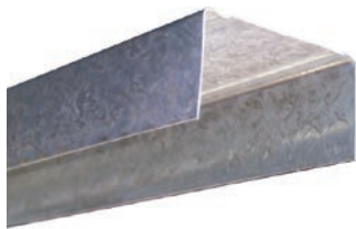
RONDO DEFLECTION HEAD TRACK 51DT75 (50mm flange) 0.75mm BMT galvanised mild steel 25mm (30mm min flange) Deflection Head Track requires special order.
