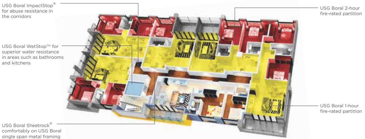
The conceptual fire safety engineering design of a typical floor in an apartment.
